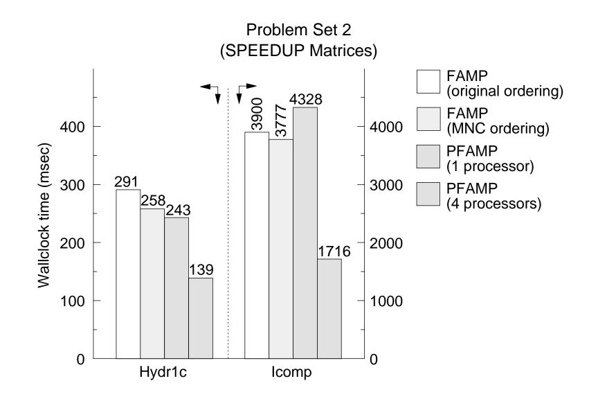
Figure 3: Comparison of FAMP and PFAMP on Problem Set 2 (SPEEDUP matrices). Note that, as indicated by the arrows, the scale of the abscissa is not the same for both problems.
