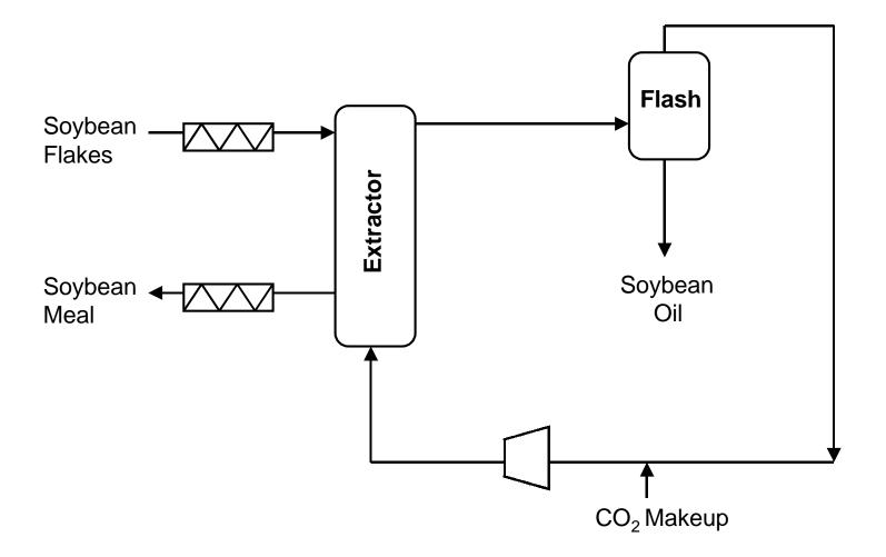
Figure 4. Process for the extraction of soybean oil using supercritical  $CO_2$ .
