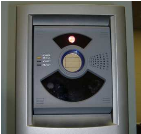
Fig. 1. The Iridian LG EOU 2200 camera used to acquire iris video sequences.
