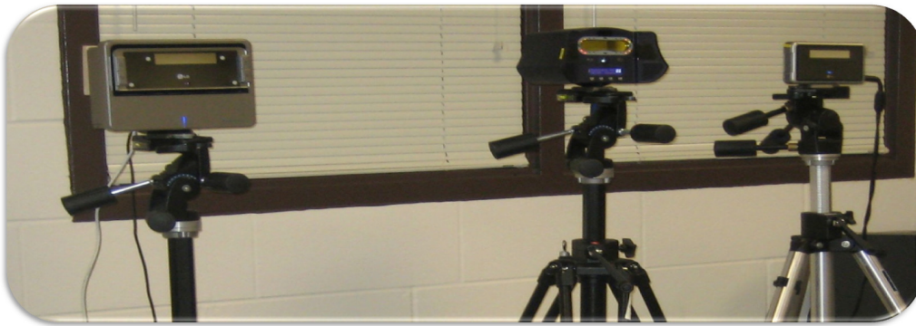
Fig. 1. Images of the three iris sensors used in this study. From left to right: the LG IrisAccess 4000, the IrisGuard AD100, and the LG TD100.
