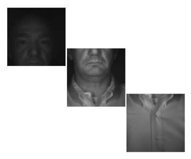
**Fig. 2** Example of corresponding frames from the IOM as the subject passes through the in-focus region of the portal. The left image shows a frame from the top camera, the middle image shows a frame from the middle camera, and the right shows a frame from the bottom camera.
