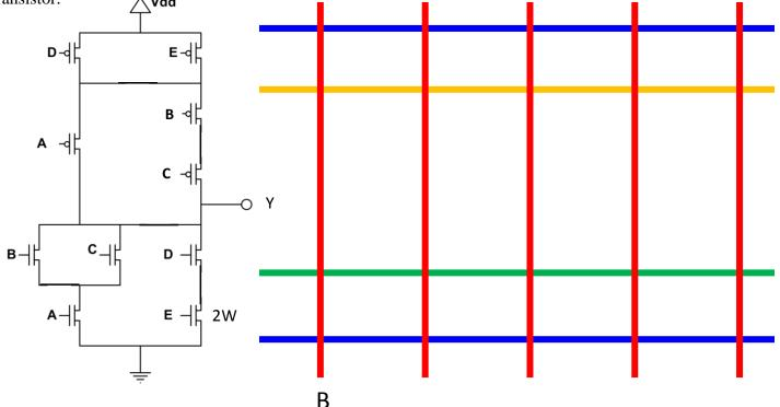
a) Annotate each transistor with a width that makes it "compatible" with transistor E's width of 2W.
