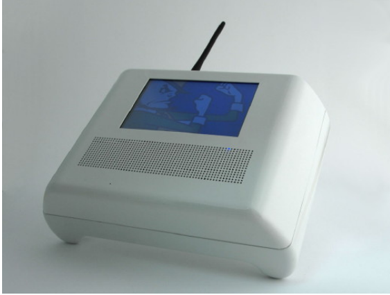
Figure 1. Highly reconfigurable portable software radio prototype implemented using open-source software and predominantly COTS hardware, providing dynamically configured multi-channel and full-duplex communications in most frequency bands from 50 MHz to 900MHz.
