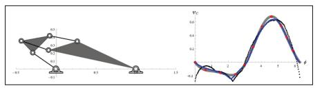
**Figure 2.** At left, a Stephenson II six-bar linkage designed to transform uniform rotation to a specific joint angle function. At right, comparing the angle of the elbow joint of a bird-wing [3] (black dots), fitted Fourier function (gray), and the function obtained from the synthesized six-bar linkage (blue) passing through 8 of the 11 task points (red dots). Both figures reprinted from [2] with permission.
