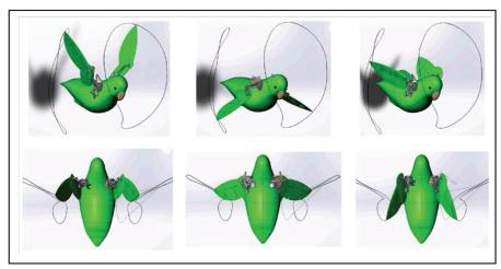
**Figure 1.** Four coordinated six-bar linkages designed to take a constant rotational input and transform it to angular outputs that match the wing movement of a bird.
