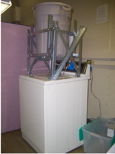
-Gray water recycling machine made from discarded washing machine
