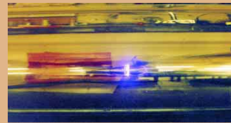
The plasma, seen here as a bright band of light, was generated by 32 pairs of electrodes placed near the tip of the nose cone.
