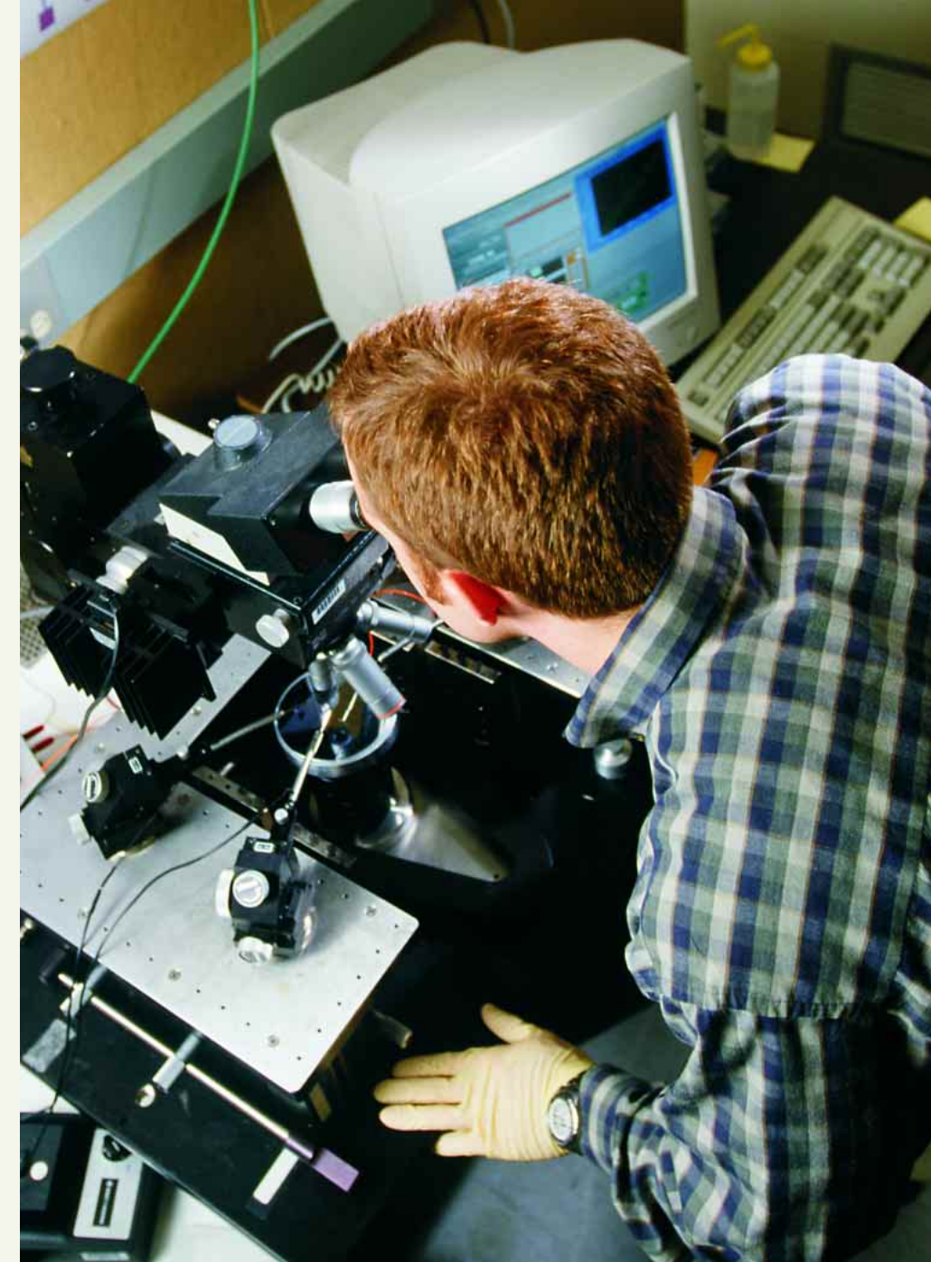
Bits-to-Chips participant Chris Russo tests a chip on the analytical probe station located within the Department of Electrical Engineering. This is the final step in the Bits-to-Chips Program.
