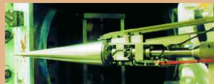
Plasma actuators were first used on this Mach 3.5 nose cone.
