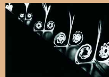
Research conducted by Robert C. Nelson and F. Payne produced these visualizations of leading-edge vortex flows.
