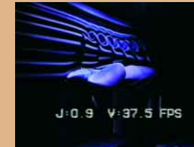
This synchronized stroboscopic smoke-flow visualization shows a three-dimensional, four-bladed propeller flow structure. The photo below shows a side view of the same visualization.
