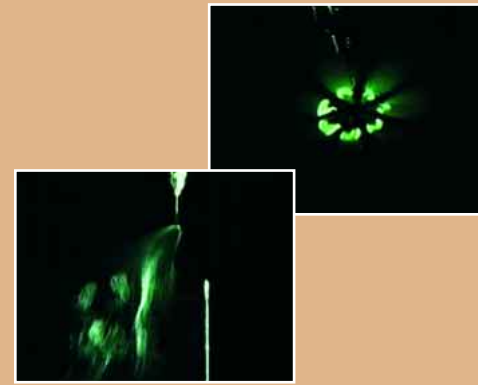
The laser light-sheet visualizations of an electrically charged microdroplet spray, shown here — a top view, right, and side view, left — employ a two-component Phase Doppler Particle Analyzer and a Particle Counter Sizer Velocimeter to capture particle velocity, concentration, and size. This helps characterize the motion of individual microdroplets during atomization and subsequent motion in the air.
