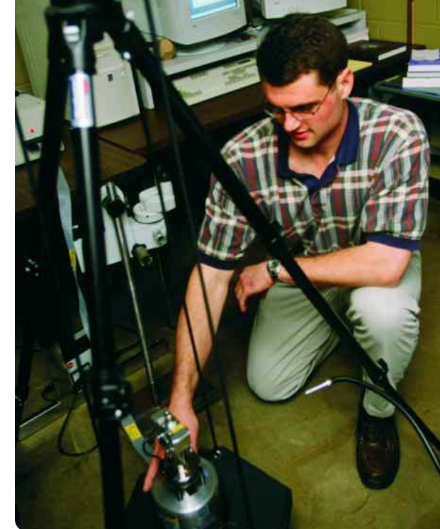
Graduate student Michael M. Crouse prepares the Department of Chemical Engineering's new atomic force microscope for the next round of readings. Although the microscope portion of this machine is standard, the ability to use the onboard potentiostat and associated software is unique.
