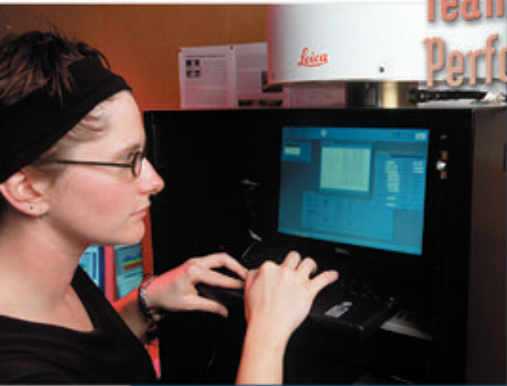
► Tracy Kijewski-Correa, monitors the static and dynamic performance of several buildings in Chicago from Notre Dame's NatHaz Modeling Laboratory. Using state-of-the-art equipment and a Global Positioning System, Notre Dame researchers are able to track the movement of individual buildings down to five millimeters with data acquired at one-tenth-of-a-second intervals. The project is funded by the National Science Foundation.
