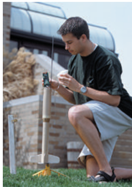
Thomas R. Szarek , a graduate student in the Department of Aerospace and Mechanical Engineering, loads a student designed microcontroller-based system into a model rocket for testing. The function of the tiny embedded system, which measures the acceleration and velocity of the rocket, is data acquisition.
