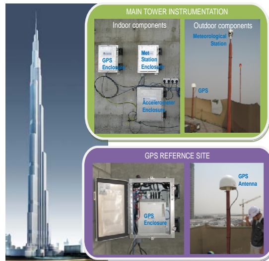
Figure 3. Schematic of SmartSync installation during construction of Burj Dubai (Khalifa), with inset photos of units as installed.
