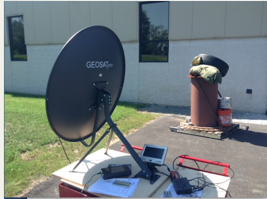
Measurement setup (above) and measured results (left) from a geosynch satellite operating at 11 GHz
