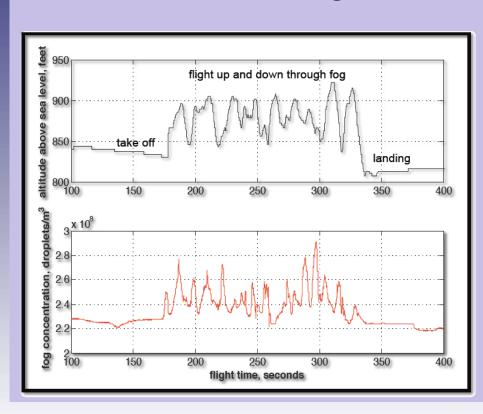
Flight altitude and fog concentration as RPV flies up and down through cloud of fog above runway.
