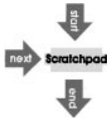
Figure 7. System defined and user defined aggregate functions are initialized with a start() call that allocates and initializes a scratchpad cell to compute the aggregate. Subsequently, the next() call is invoked for each value to be aggregated. Finally, the end() call computes the aggregate from the scratchpad values, deallocates the scratchpad and returns the result.
