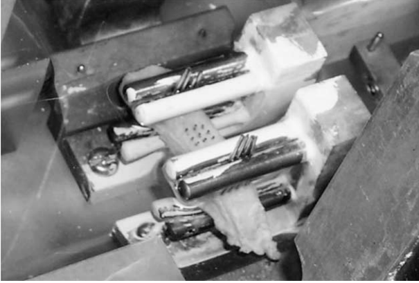
Fig. 3. Stress and strains were measured with custom test apparatus. Pin configuration II is shown.
