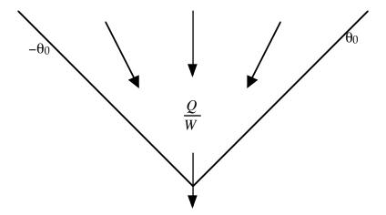
2. Film Drainage Flows: In this problem we examine the problem of drainage from a cylinder of radius R coated with a layer of fluid of density  $\rho$  and viscosity  $\mu$ , and with initial thickness  $\delta_0 <<$  R. We wish to determine the evolution of the thickness of the layer as a function of  $\theta$  and t.
