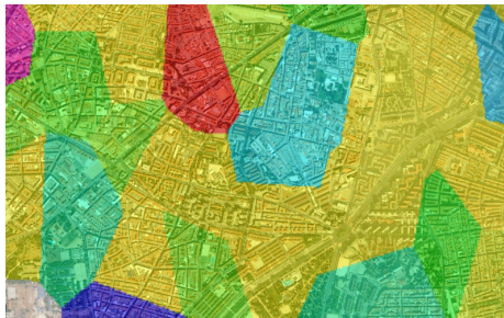
Figure: Cell Phone activity aggregated at tower level and overlaid on a satellite image. Satellite imagery courtesy Google Earth.
