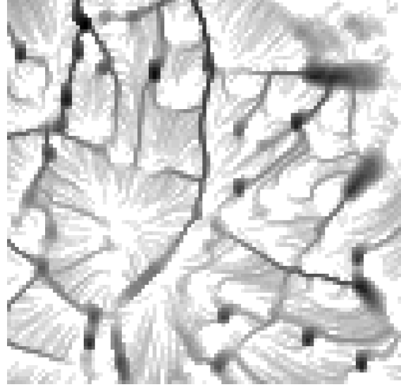
(b) Predictive elevation field. This map was generated by our inference technique acting on the cell data produced using Figure 3(a).
