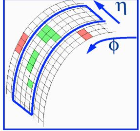
Electrons brem in tracker material and bend in  $\phi$  in 4T mag field so cluster energy is distributed in  $\phi$ .
