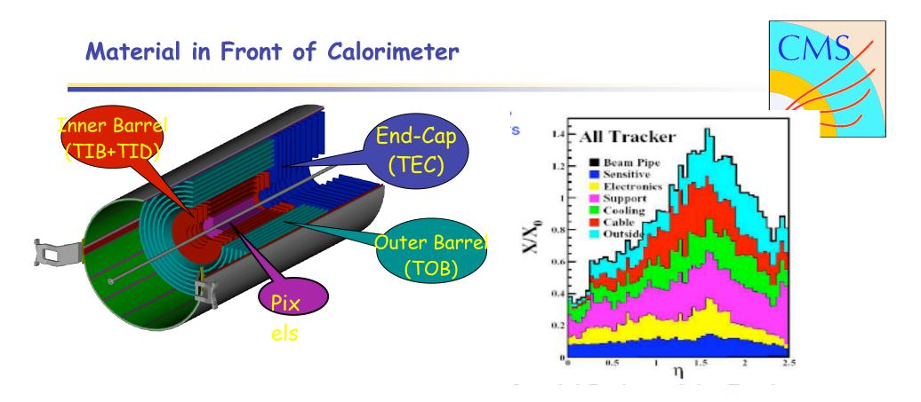
Unusually large amount of material in front of Calorimeter (0.4 to 1.4  $X_0)$  from Silicon tracker (c.f. BaBar 0.4  $X_0$  )
