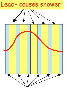
Active Detector (ionization chamber or scintillator) to measure total track length L
