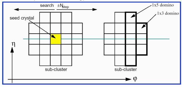
Recover Brem by making "superclusters" which are a cluster of clusters in  $\boldsymbol{\varphi}.$
