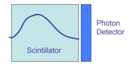
Scintillator both causes shower and is active detector
