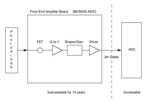
Figure 1: Schematic of front end Readout.
