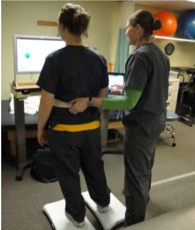
Fig. 1. Two therapists demonstrating the WeHab system. The program is run on a laptop while the main view is shown on a separate monitor. Using a Wii remote, the therapist is able to control the program.
