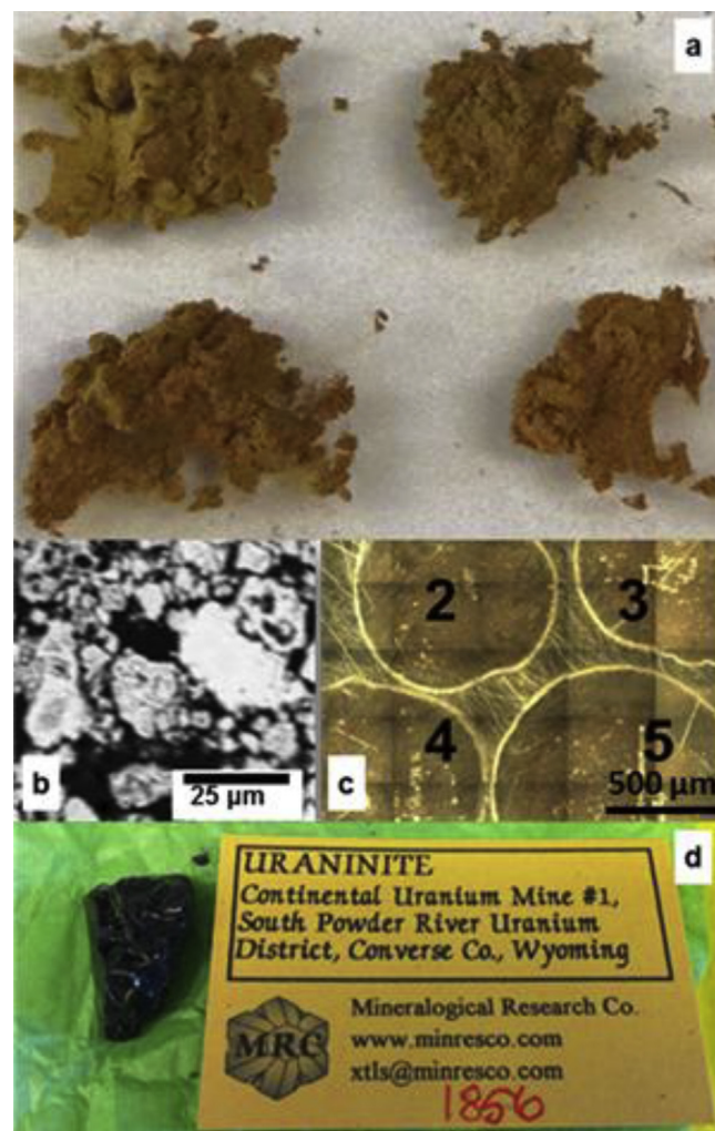
Fig. 1. (a) Photos depicting uranium ore concentrate powders. Clockwise from top left: sample 2, sample 3, sample 4, sample 5. (b) Backscatter electron image of polished epoxy-mounted uranium ore concentrate (UOC) powder. Grains are inhomogeneous with respect to size and composition as shown by variations in brightness corresponding to non-uniform distribution of U. (c) Epoxy-mounted UOC powder. (d) Uraninite from the Powder River Basin U district.
