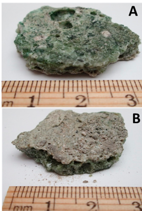
Figure 1. Samples of trinitite with the top image (A) illustrating the melted surface, whereas (B) displays a sandy bottom characterized by loosely bound materials.
