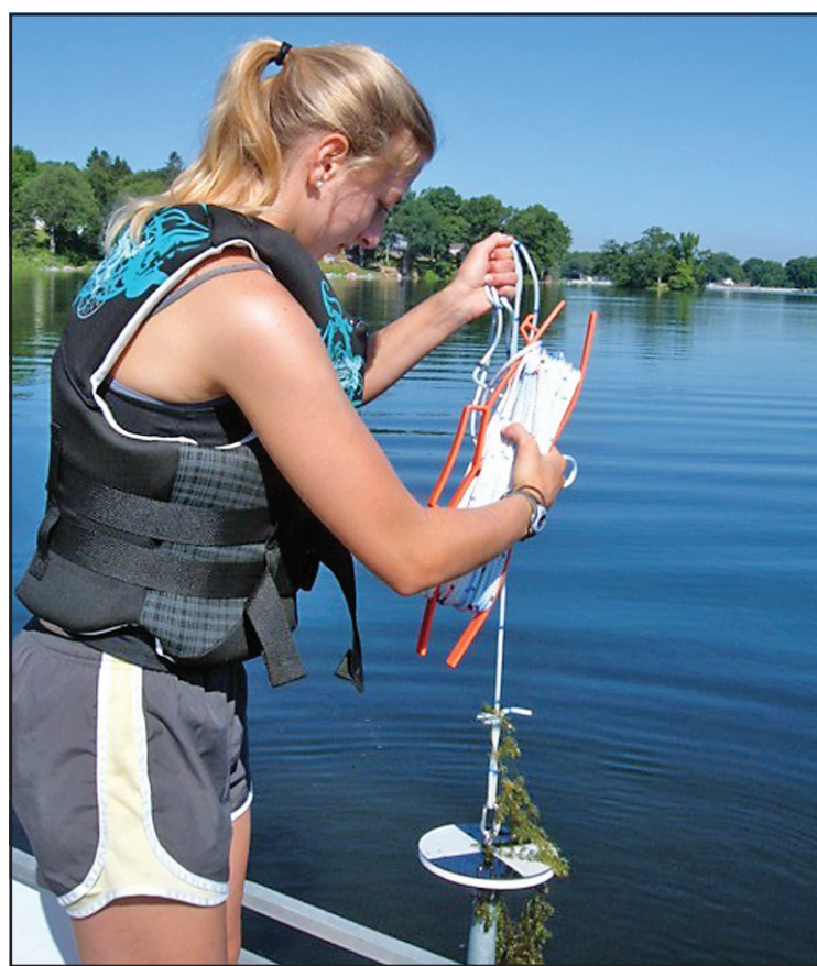
TESTING CLARITY Lowering a secchi disc until she cannot see it any more, Hannah Becker runs a turbidity test for water clarity. The rope is marked off at each meter and at 1/10th of a meter at the end to determine depth.
