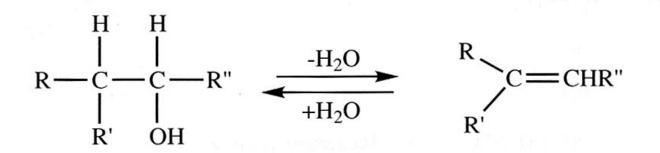
SCHEME 10.1 Reactions catalyzed by dehydratases and hydratases.
