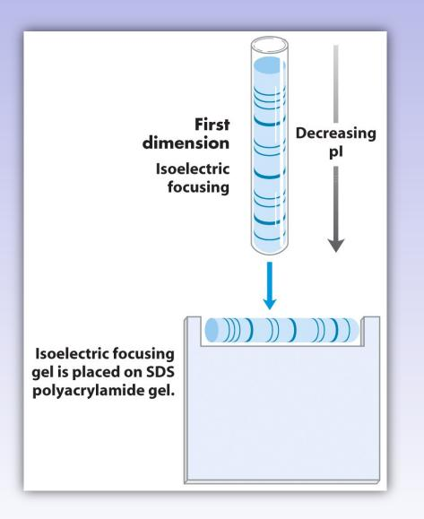
Two-dimensional gel electrophoresis
