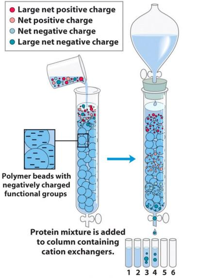
Proteins move through the column at rates determined by their net charge at the pH being used. With cation exchangers, proteins with a more negative net charge move faster and elute earlier.
