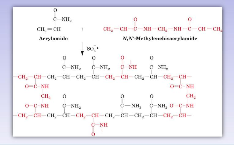
Polymerization of acrylamide and N,N'-methylenebisacrylamide to form a cross-linked polyacrylamide gel for electrophoresis (PAGE)
