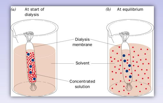
Use of dialysis to separate small and large molecules; commonly used for desalting a protein solution; dialysis tubing can be purchased with different molecular weight cutoffs
