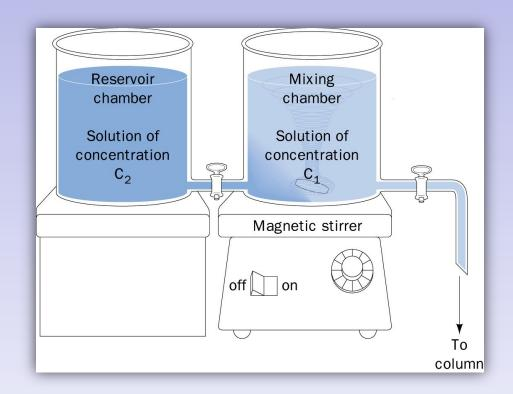
An alternative to stepwise elution. Experimental setup to generate a linear concentration gradient; non-linear and complex gradients can also generated, usually with an electronic gradient-maker.
