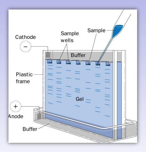
Apparatus for slab gel electrophoresis
