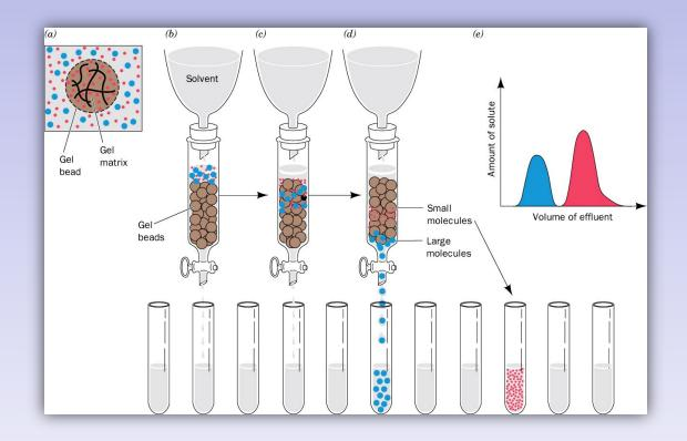
Gel filtration (size-exclusion) chromatography (GFC; SEC). Separation of proteins based predominantly on differences in molecular mass (size), with a secondary dependence on shape
