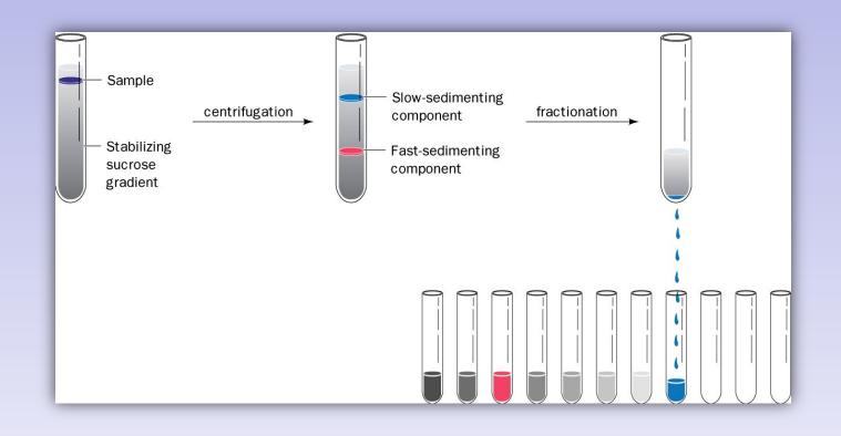
Zonal ultracentrifugation: uses a preformed sucrose density gradient. This method separates similarly shaped macromolecules largely on the basis of their molecular masses (differing sedimentation coefficients).
