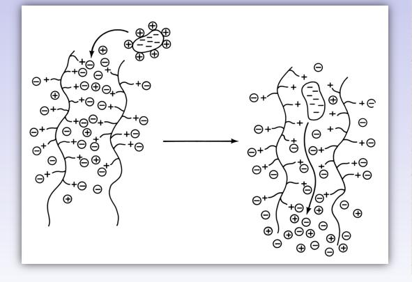
Illustration of the " ionexchange" that occurs when a negatively charged protein adsorbs to an anion exchange resin. Seven positively charged ions (e.g., HTris +) associated with the protein molecule are displaced, together with seven negative ions (Cl-) from the exchange resin.
