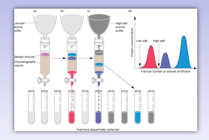
**Ion-exchange chromatography with stepwise elution**. Separation of proteins based mainly on differences in their charge properties
