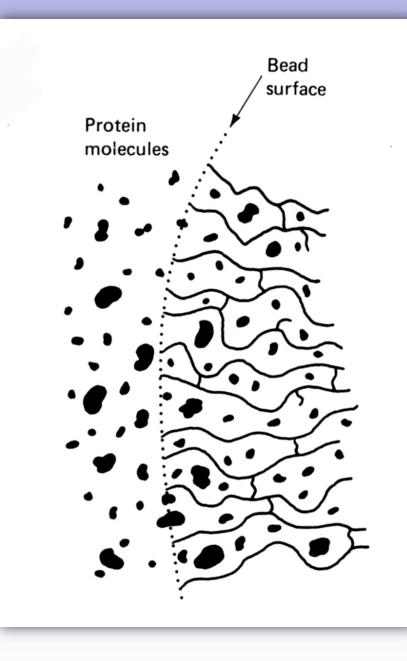
In SEC, inaccessibility of solutes to the gel may be due to the fact that a particular pore is too narrow for the molecules to pass down, or that even if large enough, there is no channel from the surface by which it can be reached.
