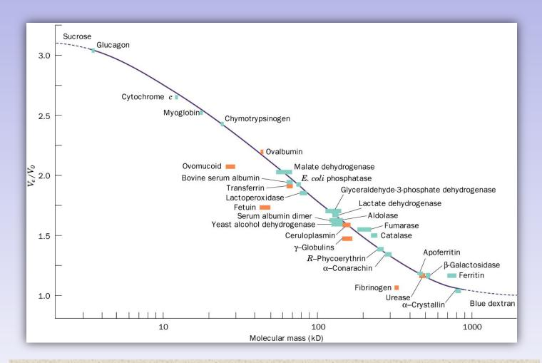
A molecular mass determination by SEC; plot of  $V_e/V_o$ against log *M* yields a highly "linear" standard curve; *M* is normally determined via HPLC using an array of standard proteins of known molecular mass
