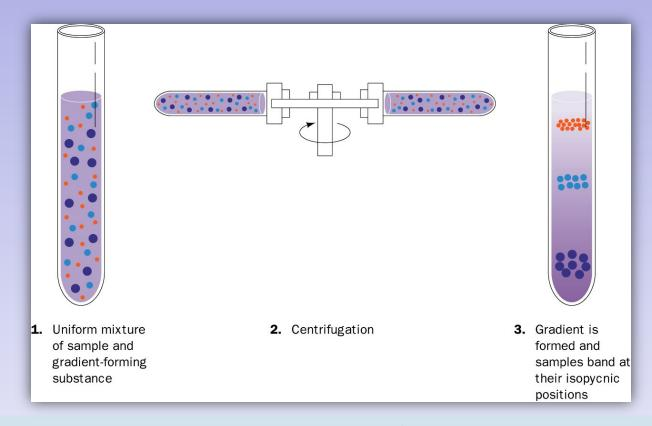
**Isopycnic ultracentrifugation** (equilibrium density gradient ultracentrifugation): Separates particles according to their densities. *CsCl* or *Cs*<sub>2</sub>*SO*<sub>4</sub> solutions are spun at high speed to create a density gradient. Sample components band at positions where their densities equal that of the solution. Used for fractionation of **subcellular organelles**, not for fractionation of protein mixtures (proteins have similar densities)
