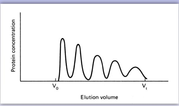
Ideal separation of five proteins, molecular weights differing each by a factor of 2, on an SE column. The same amount of each protein was applied to the column; the peak heights decrease because of the greater diffusion of the smaller molecules.
