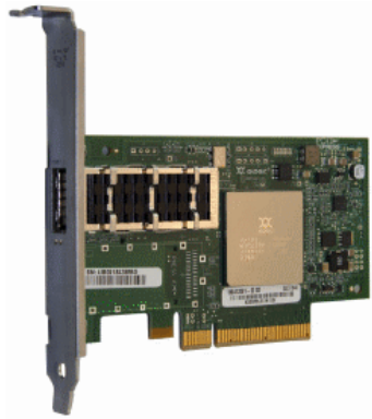
Adapter card: Processing node's link to interconnect
