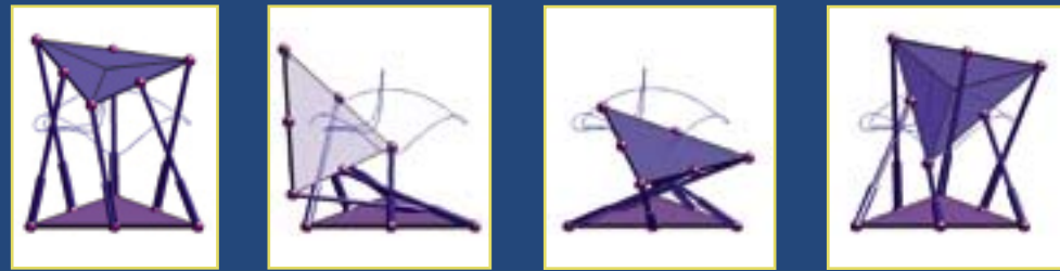
This mechanism consists of a moving upper triangle supported over a stationary lower triangle by six telescoping struts, with ball joints where the struts meet the triangles. A general mechanism of this type is a rigid structure when the strut lengths are held
