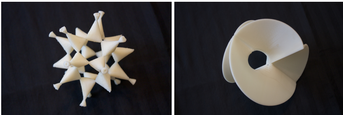
Figure 9: Photographs of 3D prints of Bertini_real decompositions. Left: Solitude. Right: the Barth Sextic. Both from a U-Print using dissolvable support material.
