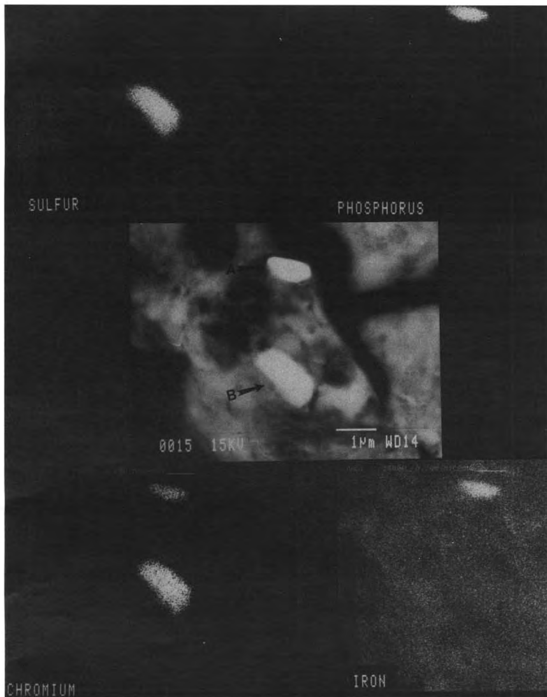
FIG. 7. Chromium-sulfur-rich and Cr-P-rich grains in Orgueil. Compare to Fig. 6.
