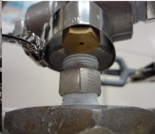
Figures 12 & 13) photos of noise source LEFT: entire unit shown clamped to vessel RIGHT: orifice on cap shown, directing air flow towards the top surface of vessel
