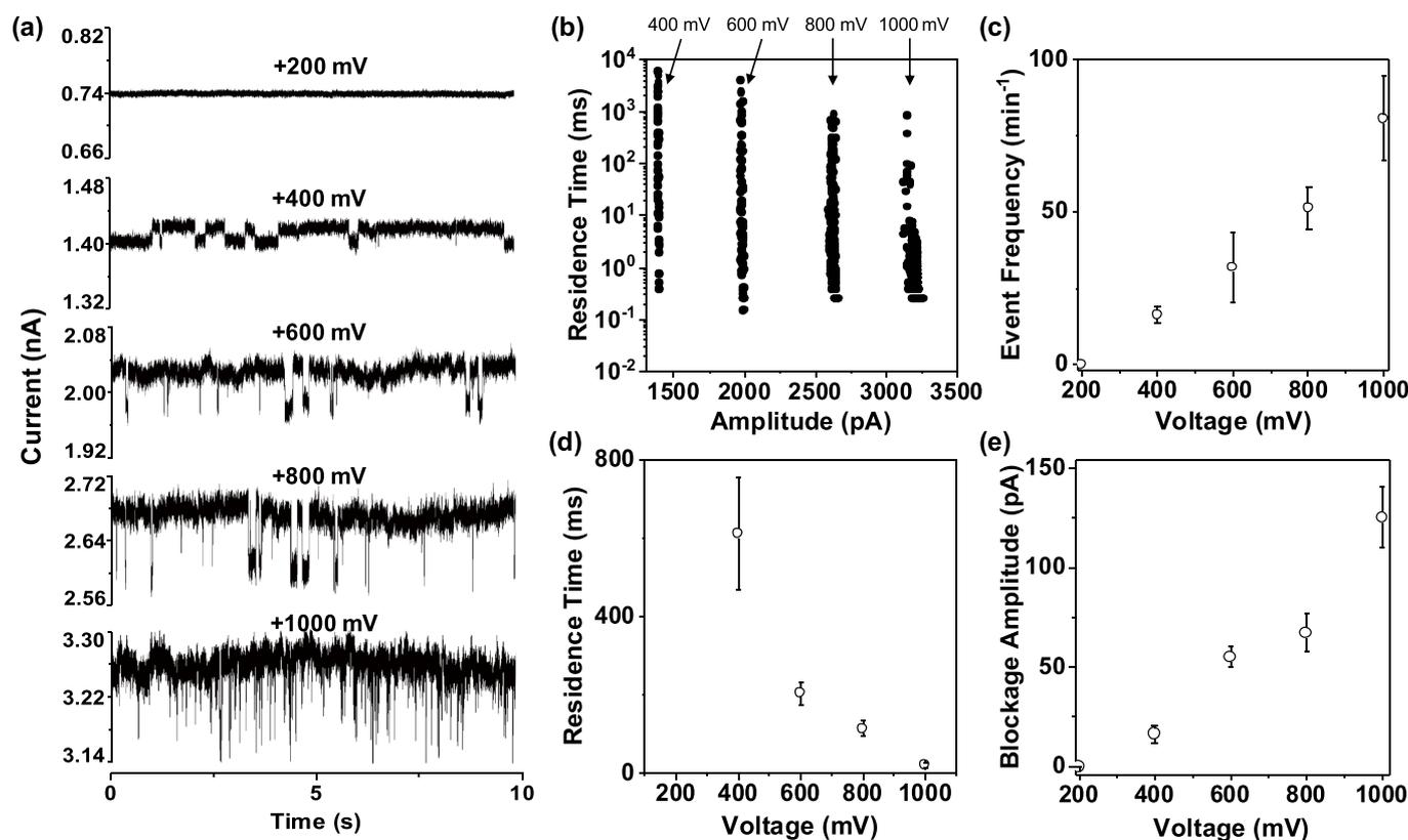
**Fig. 4.** Effect of voltage on detection of HIV-1 protease in the modified PET nanopore. a) Typical 10-s trace segments at various applied voltages; b) the corresponding scatter plots of event residence time vs current blockage amplitude; and plots of c) event frequency, d) residence time and e) blockage amplitude as a function of applied potential. The experiments were performed in a solution comprising 1 M KCl and 10 mM Tris (pH 7.5). The concentration of HIV-1 protease used was 100 ng/mL.
