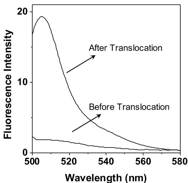
**Fig. 3.** Fluorescence intensity of the nanopore tip-side compartment solution before and after 3-h eGFP translocation in the modified PET nanopore. The experiment was performed at +800 mV with 100 ng/mL of eGFP added to the base side of the modified nanopore bathed in a pH 5.0 electrolyte solution comprising 1 M KCl and 10 mM Tris. The fluorescence spectrum was obtained with  $\lambda_{\text{ex/em}} = 488/507$  nm at room temperature.
