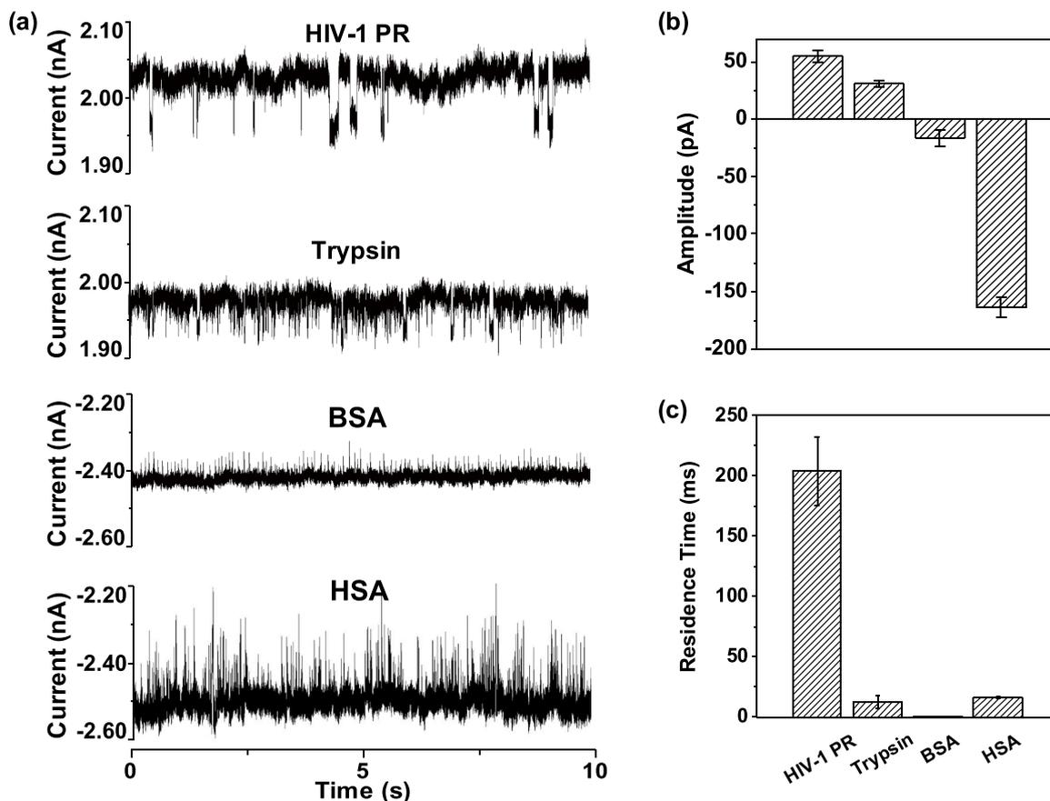
Fig. 5. Differentiation and characterization of proteins in the modified PET nanopore. a) Typical trace segments of various proteins in the PET nanopore, and their corresponding event mean (b) blockage amplitude and (c) residence time plots. The experiments were performed at (+)/(–) 600 mV in a solution comprising 1 M KCl and 10 mM Tris (pH 7.5).
