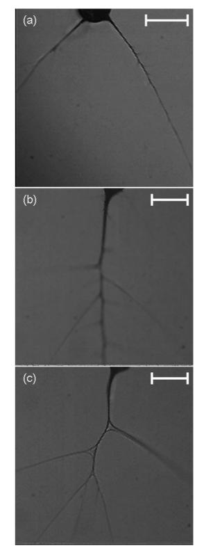
Figure 6. Images of the electrospinning jet emerging from the meniscus, scale bars: 300  $\mu m.$  a) Two jets emerging from the meniscus forming multiple fibers out of the same meniscus. b) A single jet branching out to form a vein-like structure in the fibers. c) Higher order branching of the fibers.
