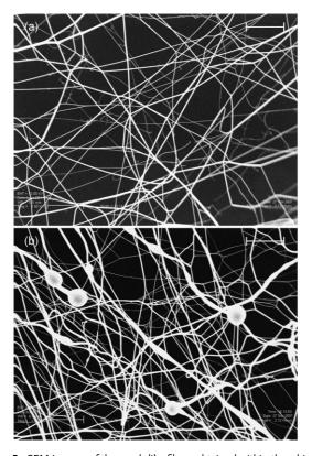
**Figure 5.** SEM images of the mesh-like fibers obtained within the whipping zone at 3.3 kV at different frequencies, scale bars:  $10\,\mu$ m. a) 50 Hz. b) 300 Hz. Increase in bead formation and thicker fibers are seen at higher frequencies.
