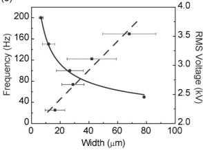
**Figure 3.** SEM images of threads consisting of multiple strands obtained at different voltages and frequencies, scale bar:  $10\,\mu$ m. a) 2.23 kV, 50 Hz; b) 3.33 kV, 50 Hz; c) 3.33 kV, 100 Hz; d) 3.33 kV, 150 Hz. Number of strands increase with frequency and decrease with voltage. e) Variation of net thread width with frequency (purple) and voltage (blue). An inverse trend with frequency and a linear trend with voltage are clearly seen.
