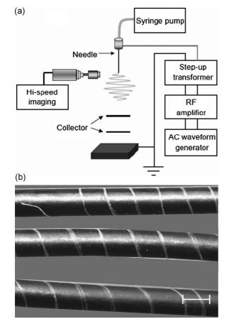
**Figure 1.** a) Schematic of the AC electrospinning experimental setup: the high voltage terminal from the step-up transformer is connected to the spinning needle, and the ground connection to a flat ground electrode. Collectors are placed between the needle and the ground electrode. b) Electrospun thread woven around a flexible cable, scale bar: 5 mm.
