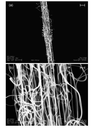
**Figure 2.** Thread morphology formed with AC electrospinning by applying a frequency of 50 Hz at a voltage of 3.3 kV<sub>RMS</sub> at a flow rate of 0.3 mL h<sup>-1</sup>. a) SEM image of the thread, scale bar: 20  $\mu$ m. b) A blow-up of the dashed square in (a). The thread is seen to be composed of sub-micrometer fibers that are intricately bound together. The nanofibers are not just woven together but are actually connected, scale bar: 2  $\mu$ m.
