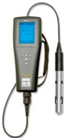
Figure 12. The Pro 20 as well as the Pro Plus can be outfitted with a polarographic or galvanic sensor.
