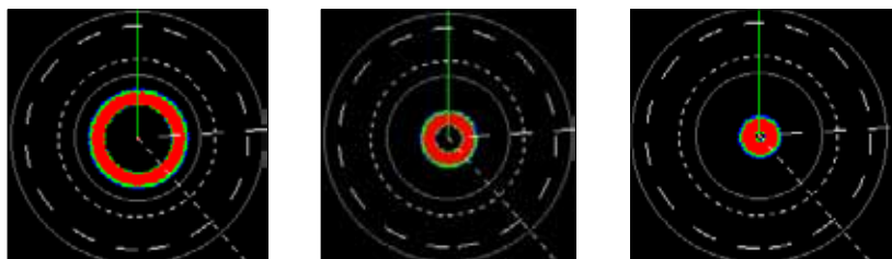
Range Offset Sequence. The circle shrinks as range is increased.
